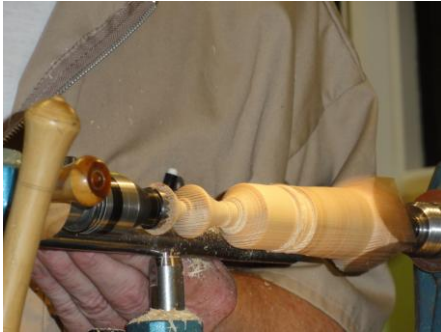
Preparing a box lid with spindle end and using a modified skew chisel
