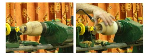
The aim, of course, is to match the outer curve of the main bowl through the underside. The splayed hollow cylinder will be the legs after cutting. It is advisable to go for three legs as these will always 'sit'. Four might look better but the finished bowl usually has a wobble.
