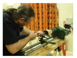
Mark switched to a hollowing out tool - a 'munroe'. Work down in stages so you can check the wall thickness. Check that the wall thickness is consistent, as this can avoid splitting as the wood dries out. In our demo it did split and had to be wrapped with masking tape. This hiccough meant that support for the next stage might be a bit dodgy. So Mark used a golf ball to give that bit of extra help in holding the bowl whilst the inside is cut away.
