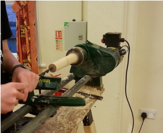
Drilling the hole
