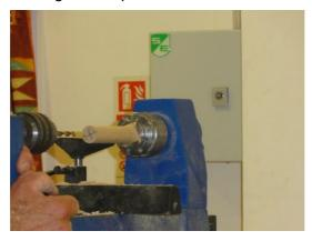
Start with what is really a very thick dowel about 8cm long. Drill out a hole for an insert which will come from a say 7mm diam. dowel. This
