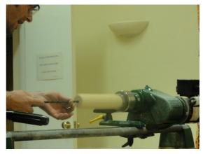
Drilling out hole in stem
