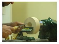
Hollowing out for cable loop
