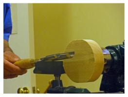
Roughing out chisels and starting block
