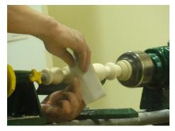
At this stage do not curve the shape just cut to the critical dimensions so you have the necks in the right place and right diameter. Richard used his skew chisel to shape up the stem but he felt most members would use a spindle gouge. He recommended cutting the beads first then the coves. This usually gives a better result.
