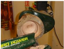
Glen Teagle made the hollowing tool Nick used on the night. It shapes by cutting very narrow ribbons . When the edge of the cutter gets blunt you just move it round a fraction. There are many similar hollowing tools on the market.
