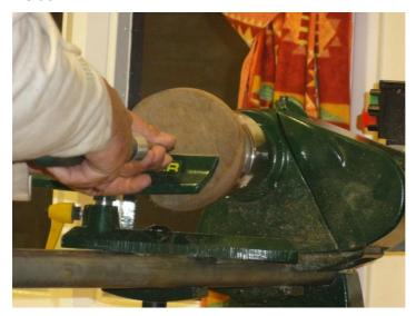
With the inside work it pays to drill out to the final depth first. You can do this as shown above with a spindle gouge using it more or less as a drill.
