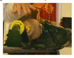
Nick was using a screw chuck which on this occasion took two of us to release it. Also note that care needs to be taken when stripping off the bark as this has a tendency to come off in chunks.
