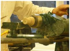
What Nick demonstrated was to turn a simple bobbin with a central hole through the middle. The two edges or rims needed to be serrated. Leaving them smooth would mean the 'tank' just skidded on one spot.
