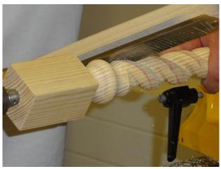
In the picture the larger microplane is being used to ease over the curves. You could use a Surform, both the flat and curved versions, but Richard felt these had too big a cutting face and tended to rip rather than shape the piece.
