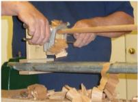
Whilst these back support stems can be turned; as you would a walking stick say, it is far easier to use a special tool. This is rather like a spoke shave which you push along the wood. There are several sizes which allow you to gradually reduce the diameter.
