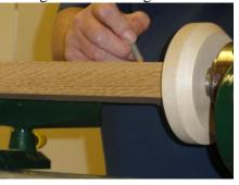
Mark out a pattern stick with each end of the curves on the master. Mick uses a skew to make the initial cuts. If you are going to have square ends then these need to be made first and delicately. Note in the right hand picture above the chuck being used has a square hole in the wood block with a screw plate attaching it to the actual chuck.
