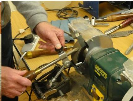
*The jig for gouges to allow you to swing the tool*
