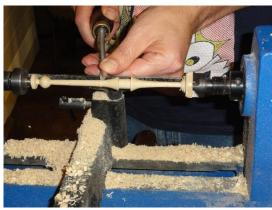
John working on the grooves on the pendant part. Note the centre is not quite down to size. This is where John used a spanner of the right size to make the final adjustment.
