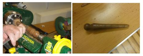
Four different turners each using a skew in a slightly different way and the fourth picture shows the finished garden dibber all done with a skew starting with a rectangular block.
