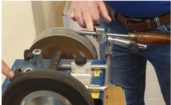
The Tormek runs a water cooled system, the wheel turning in a water bath, so that the bottom inch or so is in the water. A couple of points were highlighted regarding this:
