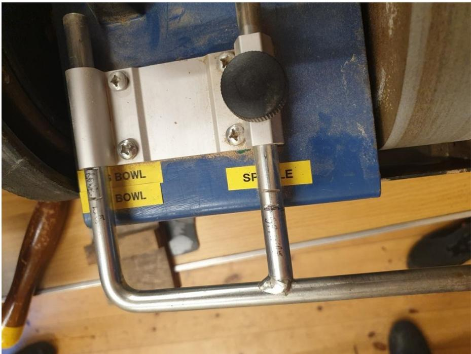
Roy has adapted his Tormek by marking the tool rest rods so that he gets the right distance from the wheel for different angles of grind for differing types of chisel.
