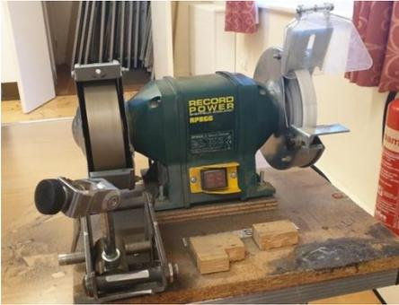
Ken brought along a Record Power grinder, which he had adapted by replacing the left hand wheel with a Cubic Boron Nitride (CBN) wheel, which can grind with less heat than a standard wheel (he got this from T&J Tools in Rugby).
