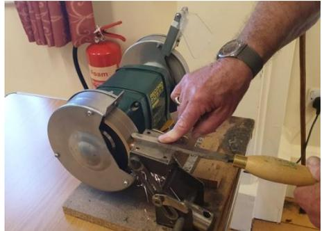
Ken demonstrated an adaptor for grinding fingernail gouges.
