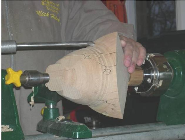
As a rule of thumb, Mick suggests that the base of the pedestal should be  $\frac{1}{3}$  of the diameter of the finished diameter of the bowl, and the pedestal height should be  $\frac{1}{2}$  the bowl diameter.
