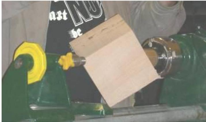
Clearly, this means that when the work piece is revolving the tips (some of which will be retained) are rather pointy, and very easily damaged by catching on tool rests, chisel digs, soft flesh etc, so great care should be taken to protect the wood from damage or unplanned colouring of the workpiece by bodily fluids.
