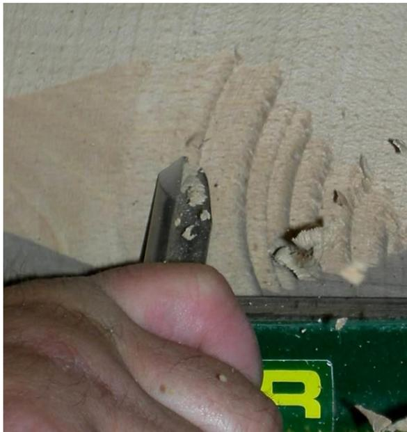
See in this photo below the angle the bowl gouge makes in relation to the cut. Yes, the wood was actually spinning!
