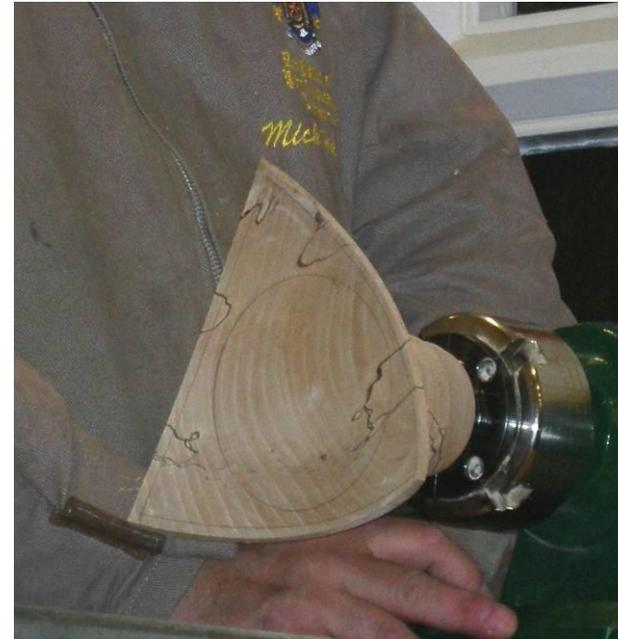
Mick uses a power sander and this can be carried out in the central area when the workpiece is spinning, but the edges should be sanded while supported from behind with the workpiece still. The piece will be finished sanded after piercing.
