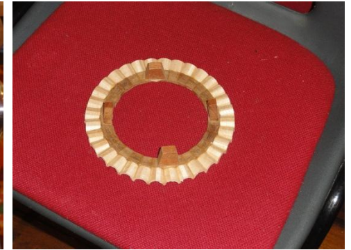
The completed top ring with a sacrificial support ring inside.
