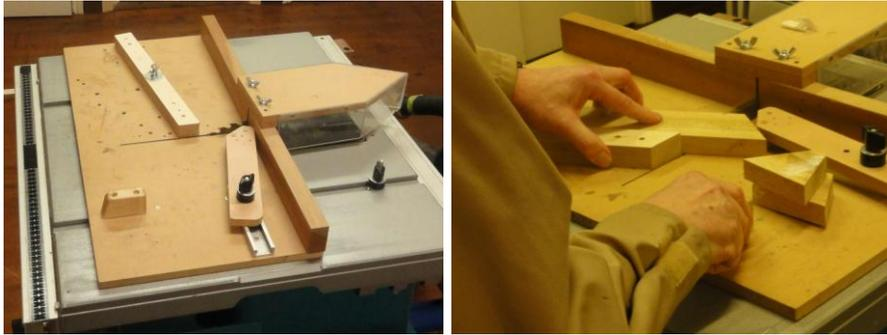
A table was given out showing the relationship between radius/number of segments/and length of cut. If using a contrasting wood spacer between the blocks this needs to be allowed for in marking up the cut line. Normally you would not taper a spacer block.
