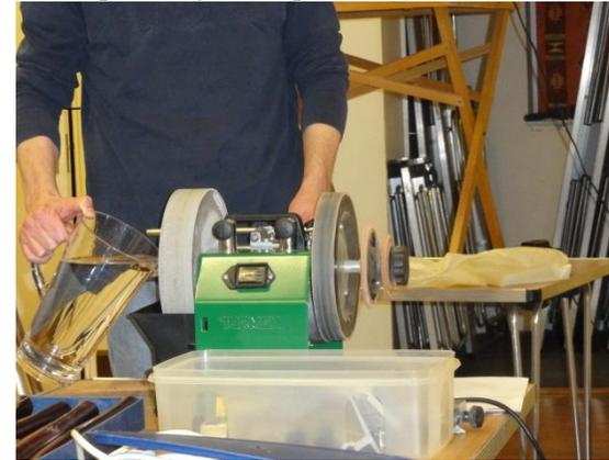
The system comes with a variety of jigs to hold whatever tool you wish to sharpen. Again this system is very workable but you do need to read the manuals so you get the jigs set up correctly.
