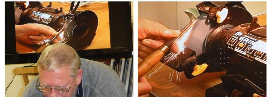
Using a spindle gouge to demonstrate Mick first grinds the end to the correct angle ( left picture above) then rolls the end gently over to give it an edge( right hand photo). With practice Mick says confidence builds and it certainly is a very quick method. Various firms make jigs to help get the angle correct. The jigs allow you to swing the gouge across the
