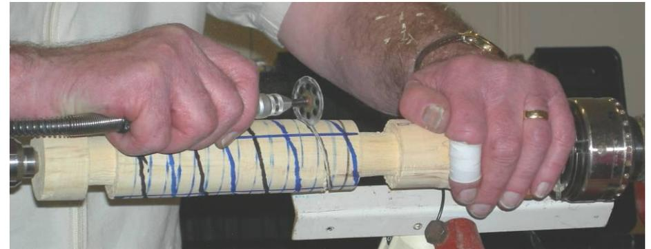
Here, the Multi-tool is used with a Dura-Grit cutter to cut the slots where the troughs will be, following your lines. Here we also see insulating tape being used to stop blood getting on the workpiece. This shouldn't be taken as compulsory equipment, though.
