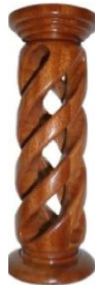
Once the full profile of the twist is complete, it can be finished by hand with sandpaper and the finish of your choice.
