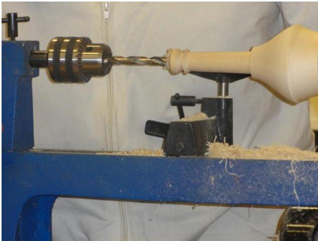
Finally the hole is drilled out. Then all that is required is to put a good finish on your Weed Pot
