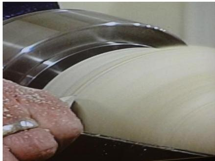
Here Ken is using the tip to start making a bead.
