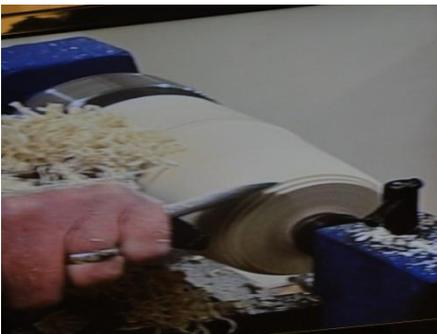
Note the angle of the cut of the skew and the cut position of the skew 1/3 down.
