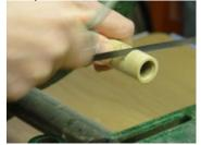
This cutting of the slot needs to be fairly accurate. A small fret saw
