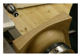
frequently to adjust the rest and also to check on the thickness of the wings (and to make sure the thickness is consistent from middle to edge). Another aside here where he mentioned that he prefers Ashley Isles chisels as they seem to keep their edge longer.
