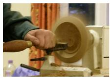
He reduced the 'island' once more and continued to cut the bowl, checking the thickness as he went, and finally removing the 'island' and finishing the bottom.
