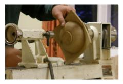
Next he needed to turn the work around again to finish the foot. For this he used a specially turned piece of wood with a felt pad glued to it. This was mounted in the chuck, and then the bowl placed over it and the tailstock secured it in place.
