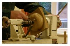
jaws, which required a flat sided tenon, and not a dovetail. It also requires a slight shoulder at the base, for which he made a special tool, ground down from a parting tool.
