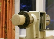
then sanded it.. The final job was to remove the 'spigot' which he did using a skew chisel, carefully finishing it by hand.
