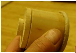
He then cleaned up the foot, by giving it a small dovetail shape using a 3/8" spindle gouge. He also reduced the thickness and
