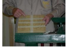
He started his demonstration by showing how a plank of ash is marked out in concentric rings. These will be cut out on the band saw with the table set at 45 degrees. He suggested using a baton on the saw to help hold the plank while you cut out the circles.
