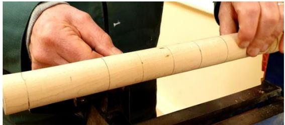
For that length it would be better to take the twist round twice, so the centre was marked at 16cm. Now, on each half, mark off a line at 4cm intervals (the narrower the gap, the finer the twist will be).
