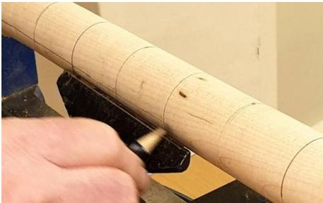
The next step is to mark 4 lines linearly along the wood, evenly spaced. You could either use the corners of the original wood square (if you haven't turned them all out), or use the chuck jaws as a guide, but they must be 90° apart. Use the tool rest as a straight edge to draw the line on
