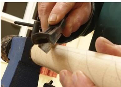
Work on the top, and gently rotate the wood, aiming for an even cut.
