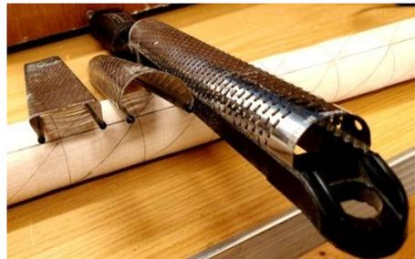
He started with a small V shaped file (he mounts them in the handle so that they cut on the pull). Follow the saw cut round, but don't go too deep to start with.
