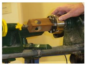
Then put dovetail on each end so you can hold it in the lathe firmly and accurately. Drill through the free ends with the holes to take the bits and pieces later.
