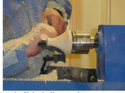
Having parted off the bullet, work can start on the base/stand. In the above photo you can see the piece is nearly formed. Before parting off the bullet part was sanded, going through the grades, and finished with "Speed and Ease".
