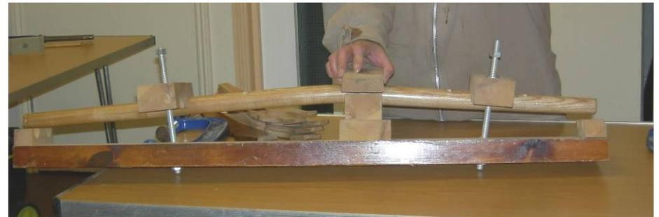
If you are forming the spindle set for the back of the chair, make sure that you glue them into position as soon as you remove them from the former, so that they restrain each other from bending back out of shape. Anne recommends Cascamite Resin Wood Glue, which I found on Amazon in various sized tubs.
