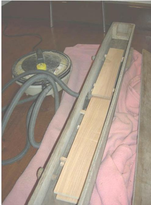
When the wood is put into the steamer box it is separated by a series of offcuts from the same type of wood, so as to allow the steam to circulate.
