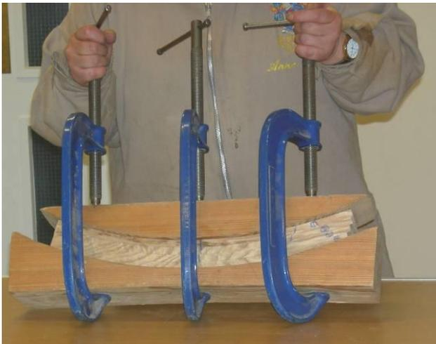
When removing the wood, your glasses will steam up instantly allowing people to sneak into the workshop and steal your biscuits, so remove your glasses. Clamp the wood into the jig as quickly as possible.
