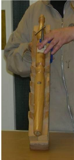
The drilling is done on a pillar drill, using a series of Vee blocks, with the workpiece clamped securely in place. Before doing the drilling, check and re-check that you are drilling the holes in the right place, as you've invested a lot of time and effort in getting the wood into shape and you wouldn't want to get it wrong, especially with ladies and small children present.
