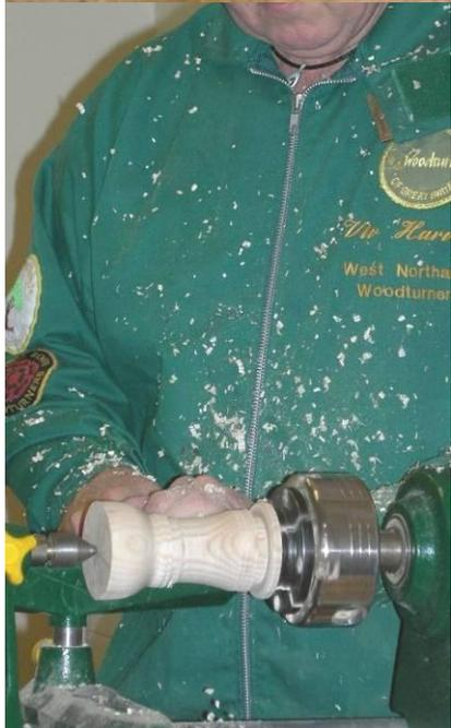
Again, Viv uses the simple route and doesn't fuff about marking out the centre of the wood, he just does it "by eye" and that's generally close enough. Once the wood was roughed out to diameter, Viv again used a parting tool to turn the spigot ready for mounting the candle sticks in the chuck.
