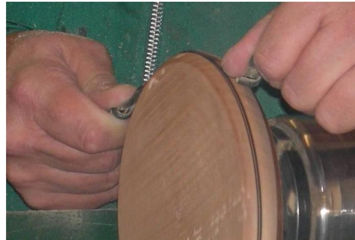
Having completed the profiling and sanding of the top face, leave the drilling of the mounting holes for the candlesticks until they have themselves been turned, as you may want to experiment with the exact placing of the candlesticks. Viv uses a 19mm Forstener bit to make these holes.
