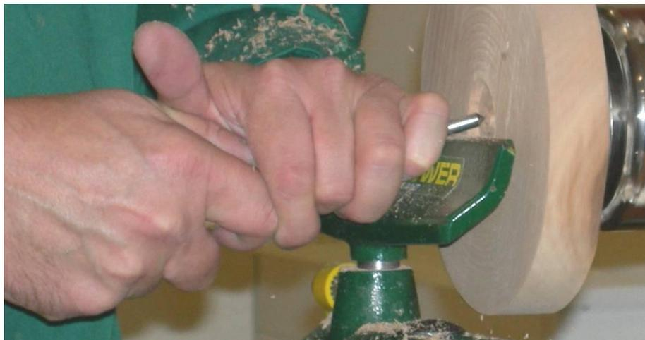
On the outside diameter Viv rounded off the bottom edge and added a lip with a skew chisel, using it as a scraper. Then the bottom of the base was sanded off initially using a disk pad (the breeze block finish) and then using 240, 320 and 400 grit Abranet, and 600 grit after a coat of sanding sealer. Viv applied friction polish as a finish, with a coating of Carnuba wax over the top.
