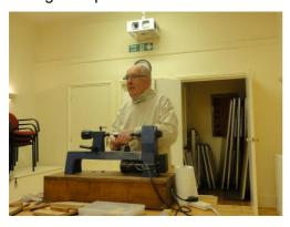
So starting with the blanks these need to be drilled out fitted onto the mandrel and turned down to the desired size. If you are using a plastic blank it pays to warm it first other wise the drilling may shatter the plastic. This is because you are turning down to a very thin tube.
