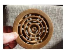
First a tea pot stand using a parting tool to cut the gooves and offset the circles on the underside. Just cut half way through.
