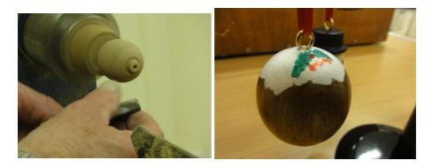
The actual process is to work up the shape , sand it then seal it using sanding sealer.
