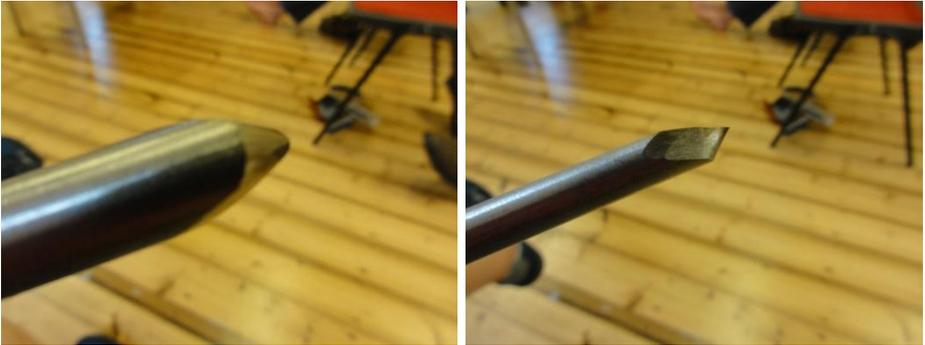
The finished spindle gouge with clean cutting edge.
