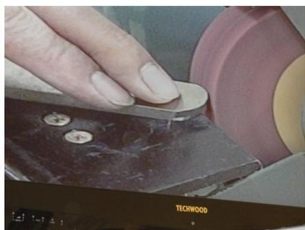
Using a platform the angle of which can be adjusted. It allows you to swing easily through the grind.
