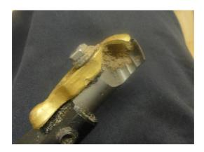
The cutter shown above is typical of the more costly tools. The cutting edge is small and there is a cover to the blade which controls the amount of cut. With nearly all these tools you cut or rather shave off small amounts but in a very controlled fashion. To sharpen the edge use a diamond sheet to put an edge back on.
