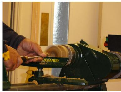
Use low speeds and ensure you have tightened the chuck as much as possible. Speed is not the essence during this stage- safety is.
