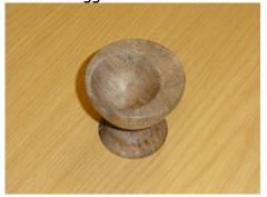
This rather simple shape is anything but simple to turn as Nick demonstrated. You need two spigots so that the chuck can get a tight grip for both operations. The first operation after the spigots being to reduce the block and form the egg cup shape.
