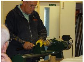
Now using the chuck alone on the smaller spigot attempt to hollow out the hole for the egg.
